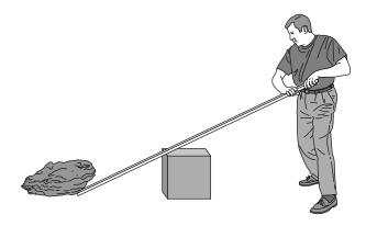
Which simple machine is the person using?
